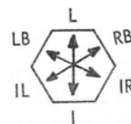
BANKING ATTITUDE CHANGES IN A HALF-ROLL MANEUVER
